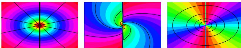
3. **A half body in two-dimensions is generated by a combination of source and uniform stream  $\Psi = Ur \sin \theta + m\theta$ .**
