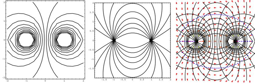
Figure 6: Potential, stream and combined contour with velocity respectively.
