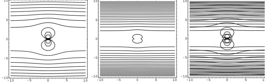
Figure 2: Comparison of doublet and calculated stream function respectively
