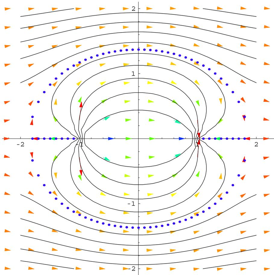
Figure 5: Streamlines and the Rankine Body with velocity field
